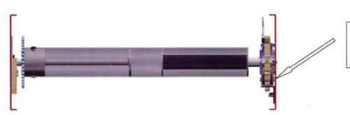
11) Secure inertia brake with one M12 bolt and nylock.
