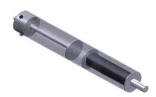
4) Insert Telescopic dummy end into the tube so that is protruding 1-2 mm, then weld.'
